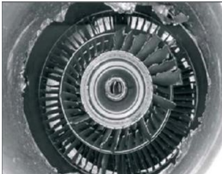
Figure 6. Jet engine blade damaged by bird strike (source, ATSB).
